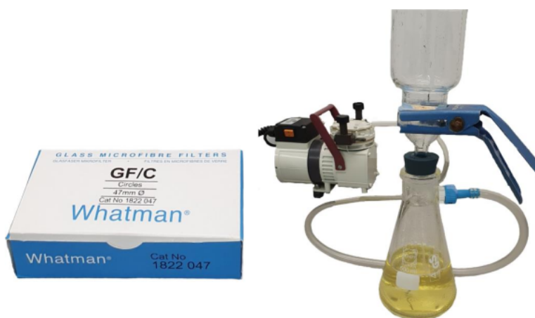
Figure 3.15 Filters and apparatus for the filtration process using a vacuum pump
