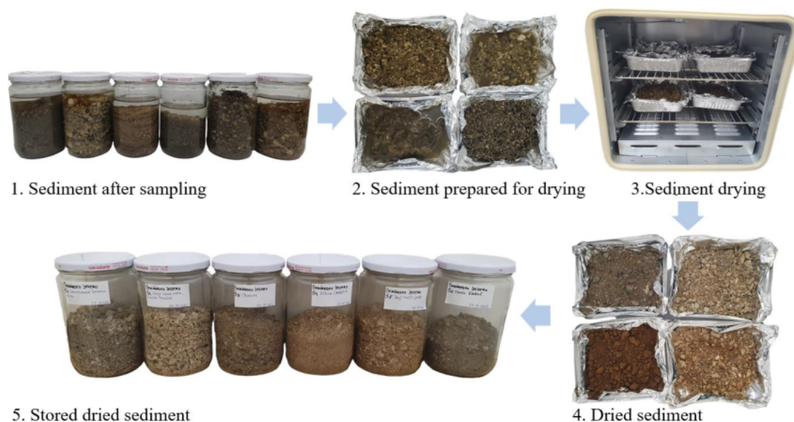
Figure 3.12 Sediment drying procedure
