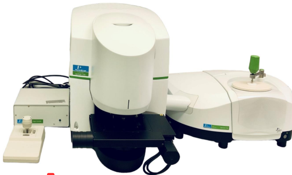
Figure 3.18 Perkin Elmer microscope Spotlight 200i with ATR FTIR Spectrum Two
